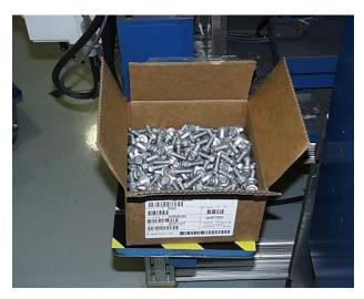
The photo above and on the left shows light-weight metal bushings. This packaging is sufficient since the parts do not weigh much and will not get damaged when packed bulk into a small carton. The carton on the right shows an example of how bolts should be shipped. This is a ¼ keg carton.
