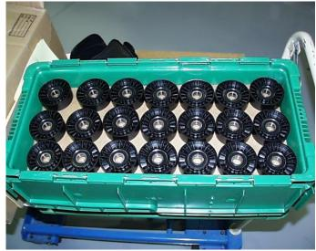
The photo above on the left shows a ribbed plastic pulley packed into a returnable container. The vertical row dividers separate each pulley's ribbed surface from being damaged. Notice also that there are two extra pulleys packed on the end of the container at 90 degrees to take up the extra slack in the container. The photo above and to the right shows a flat edge plastic pulley layer packed with 21 parts per layer. No row dividers are needed here since these pulleys do not have ribs.
