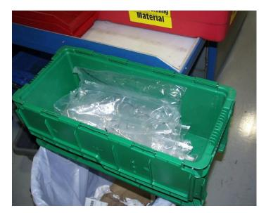
Some suppliers are required to ship small plastic parts such as bushings in plastic bags. The bags are then returned to the supplier for re-use with the empty container as shown in the photo on the left.
