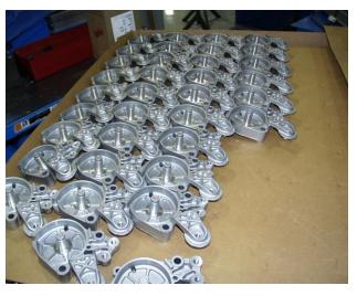
The photos above have machined surfaces and need to be layer packed as shown. These are larger sized parts that do not fit well in manually handled containers.
