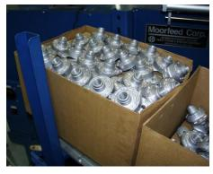
If the aluminum castings have machined surfaces, they should be divided or layer packed. In the three photos above, the one on the far left does not have any critical surfaces, so it can be "bulk packed" into the small carton. The photo in the middle has parts with machined surfaces so they are cell packed. The photo on the right shows parts that also have machined surfaces. They are layer packed and laid out in a uniform manner.
