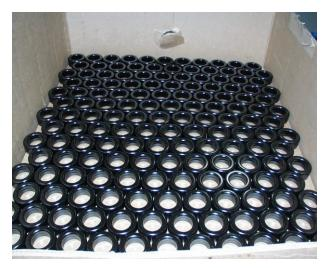
The above photo shows raw pulley shells. Raw pulley shells have a pre-operation in the MUVIQ facility and have to be handled prior to going to the production line. It is recommended that raw pulley shells be shipped in an expendable "bulk pack" in order to minimize packaging costs. Notice that they are layer packed.
