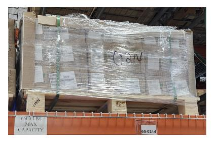
The left photos above show the Palletization layout for manually handled cartons that feature opentops. Note that the open-topped containers should be palletized with a common lid for layer separation. The pallet load should be wrapped or banded securely for part protection as shown, with corner boards to protect when stacking same as photo on the right.
