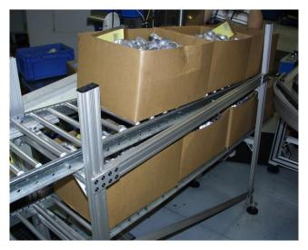
The two photos above show aluminum castings in manually handled cardboard cartons. The cartons should be open-topped as shown. The cartons in the photo on the left are a 12" X 12" X 12". This is the ideal size for aluminum castings. The photo on the right uses a 12" X 15" X 12". This is also acceptable as long as the weight is less than 30 lbs.
