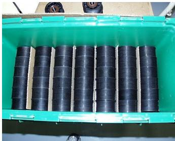
The two photos above also show plastic pulleys in returnable containers. Notice that the photo on the left shows flat edge pulleys placed in rows of 8. No vertical row dividers are needed since these pulleys have no ribs. The photo on the right shows ribbed plastic pulleys that do need row dividers to protect the ribbed edges. Note that the photos show just the first layer in the container. Most all containers will have multiple layers separated by horizontal layer dividers.
